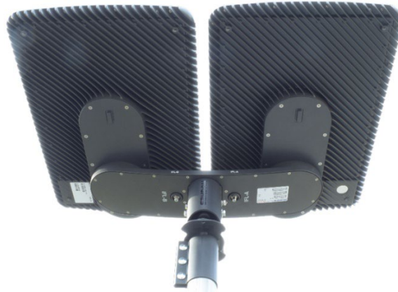
Figure 16: ODU mounted to mast adapter
