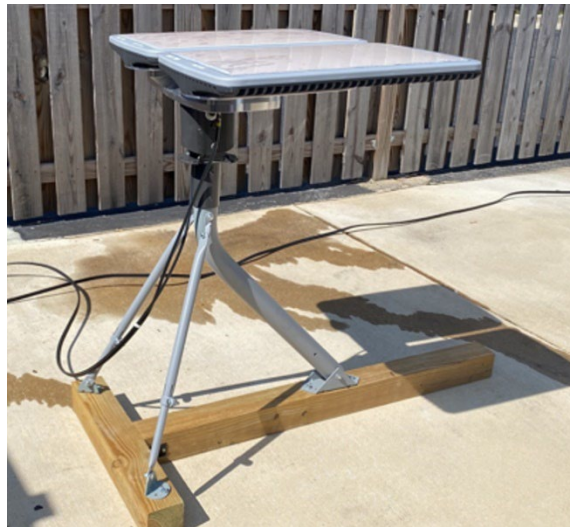
Figure 20: ODU mounted to trimast with mast adapter
